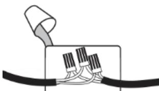
To prevent moisture penetration from conduit system or cable sleeve use potting compound in the junction box (by others) (4).
